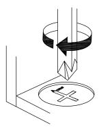
Turn cam lock clockwise to tighten.
