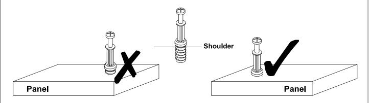
Tighten quickfit until shoulder is flush with panel. Do not overtighten or undertighten.
